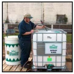
Place pick-up tube in drum of concentrate. Use air pump to transfer concentrate from drum through discharge wand.
