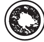
SINK OR DRAIN PIPE BUILDUP 30% FLOW
