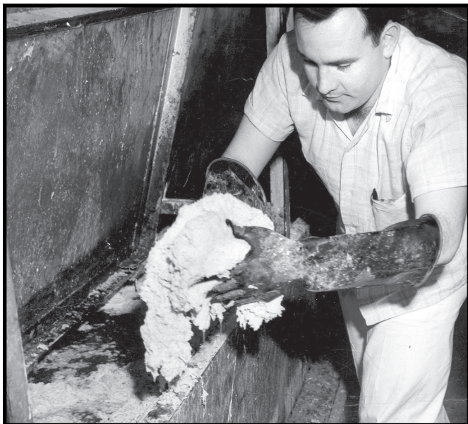
Overspray reduced to a clean buoyant mass—non-sticky; easily removed.
