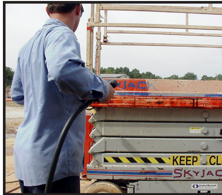
Pressure Wash After Adequate Exposure
